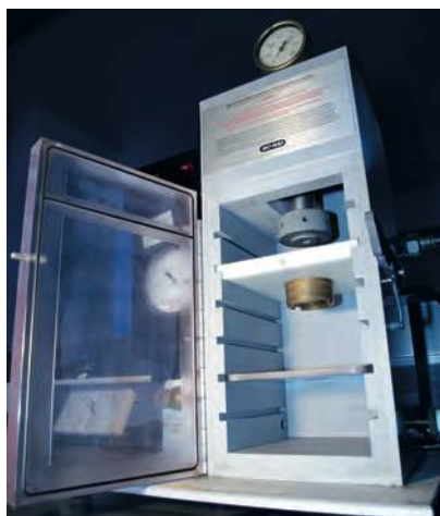
◀ A gene gun or biolistic particle delivery system is a device for injecting cells with genetic information.
